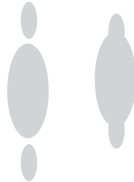
Trace of spraying a fluid at low-pressure without using air.
