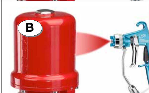
Symmetrical trace of spraying a fluid using air. No tail-end is formed.
